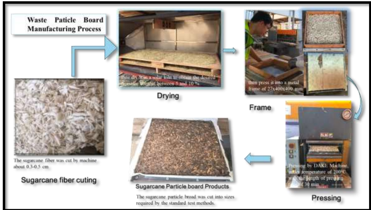
Picture1: Waste Particle Board Manufacturing Process
