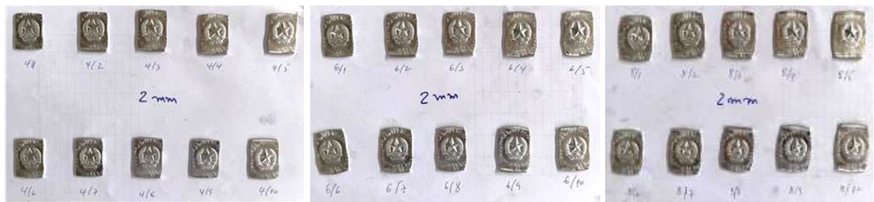
Figure 3. 30 trials for 2 mm aluminum sheets across three pressure levels (4, 6, and 8 bar)
