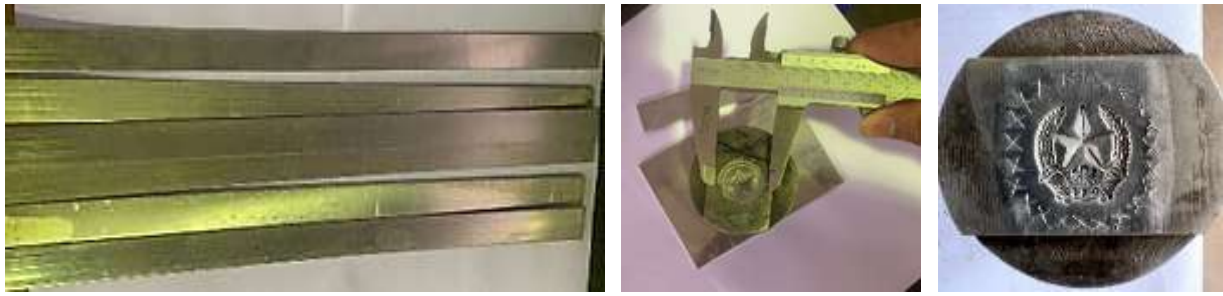
Figure 1. Aluminum sheets (99.5% purity) and the micrometer used for verifying sheet thickness (2 mm and 3 mm) before hydraulic stamping
