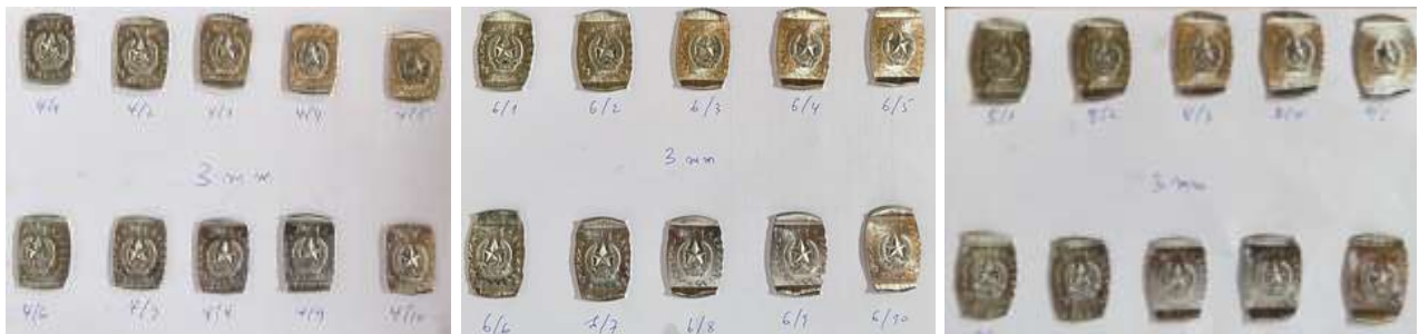
Figure 4. 30 trials for 3 mm aluminum sheets across three pressure levels (4, 6, and 8 bar)
