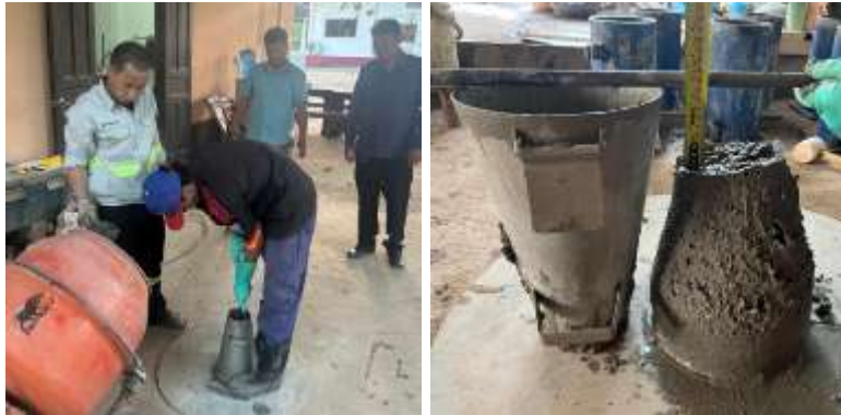
Figure 3. Testing the workability of fresh concrete
